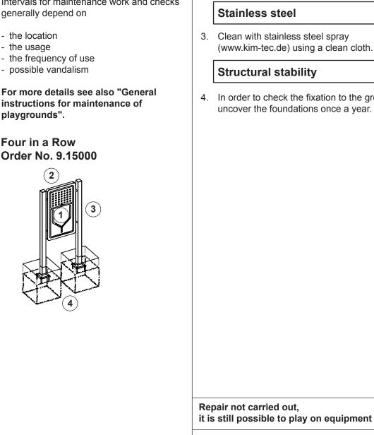
Playground equipment 1. Check that playing tokens are complete (red x 21, blue x 21) und make sure they move smoothly. 2. Check that the bolts and screws on the back and on the stand posts are tight and retighten if necessary. 3. Clean with stainless steel spray (www.kim-tec.de) using a clean cloth. 4. In order to check the fixation to the ground, uncover the foundations once a year. Special notes, e.g. for repairs
